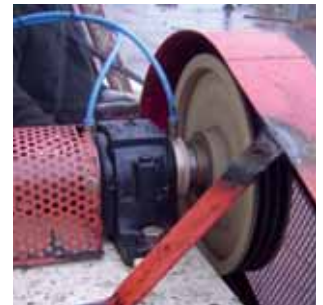
70mm LabTecta-PB™ with Air Purge installed on a centrifugal fan pillow block SKF® SNL 516-613 in Argentina (Case Ref: 3218)
